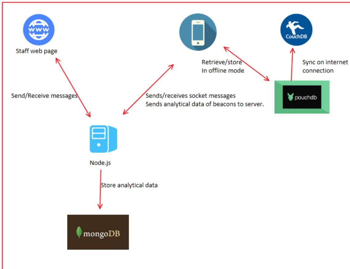
As you can see from the picture, the clients send and receive requests and answers from the mobile phone. As you can also see, client's devices send analytical data to the server. The data contains information about when client approach to a car, when client distanced the car, and what car was that. Below is the flow of Client architecture:
