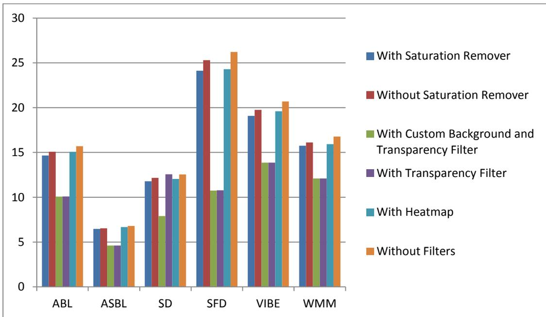
Figure 17: FPS rates comparison between algorithms and filters. Test conducted on an Orange PI.
