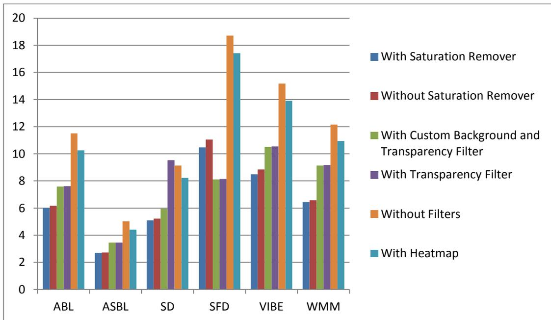
Figure 18: FPS rates comparison between algorithms and filters. Test conducted on a Banana PI.
