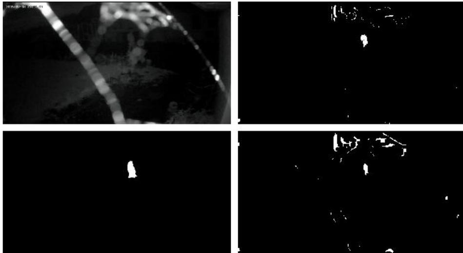
*Figure 23: Noise object suppression example (intruder present)*
