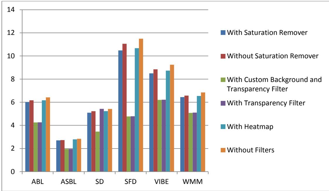
Figure 16: FPS rates comparison between algorithms and filters. Test conducted on a Raspberry PI.
