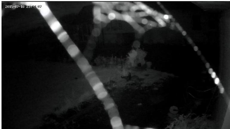
*Figure 11: Semi-transparent cobweb over saturating the frame*
