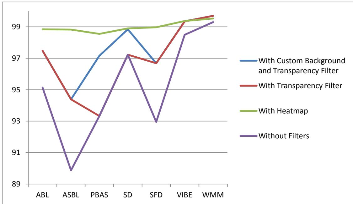
Figure 20: PCC rates achieved from feeds containing cobwebs
